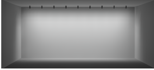
30" SETBACK / 30" ON CENTER SPACING / 10° TILT
