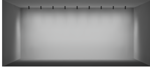
36" SETBACK / 36" ON CENTER SPACING / 15° TILT
