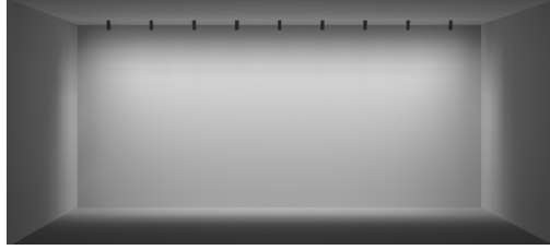
30" SETBACK / 30" ON CENTER SPACING / 10° TILT
