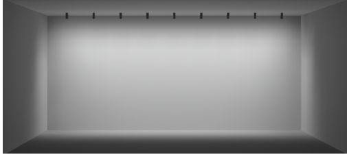
30" SETBACK / 30" ON CENTER SPACING / 10° TILT
