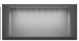
**8FT CEILING** 36" SETBACK / 36" ON CENTER SPACING / 15° TILT 36" SETBACK / 36" ON CENTER SPACING / 15° TILT 36" SETBACK / 36" ON CENTER SPACING / 15° TILT
