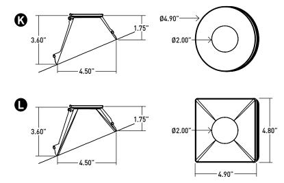
SLOPE 2 BAFFLE: 30° - 45° (7/12 - 12/12) SLOPE RANGES
