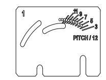
SLOPE 1 BAFFLE: 15° - 30° (3/12 - 7/12) SLOPE RANGES
