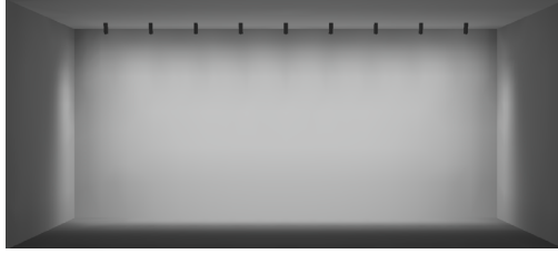
36" SETBACK / 36" ON CENTER SPACING / 15° TILT
