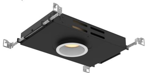
Our innovative design allows users to easily and effortlessly obtain desired light effects. Our precision machined baffles accommodate up to two effects devices, and the adjustable versions allow the user to tilt and lock the fixture from 0-40° without the need of a tool.
